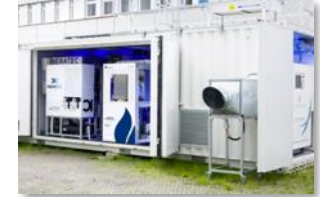
PtL-Plant with Direct Air Capture (Kopernikus Project)
